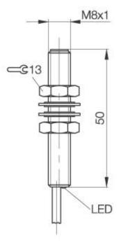
Inductive Sensors BES M08MI-PSC15B-BV02 M 8 x 50 normally-open Sn=1,5mm shielded
